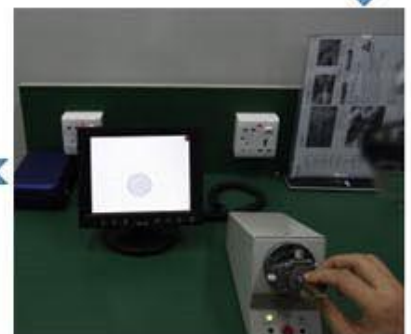
Cleaning end face
