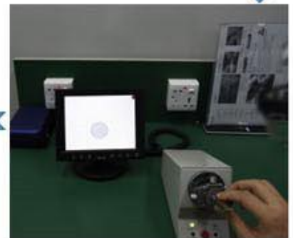
Cleaning end face
