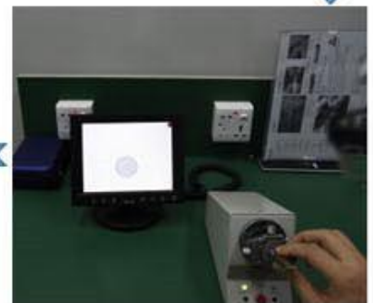
Cleaning end face
