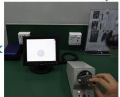
Cleaning end face
