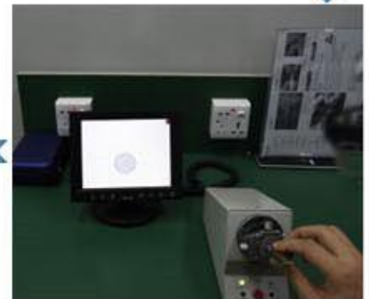
Cleaning end face
