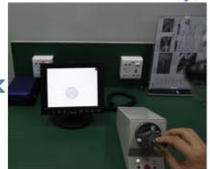
Cleaning end face
