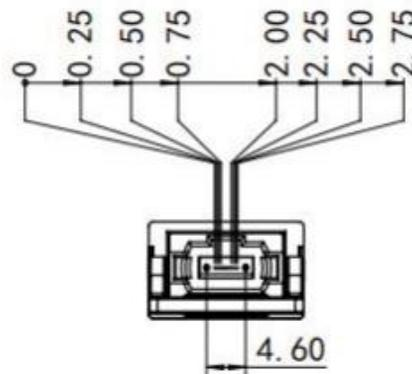
Attention: To minimize MPO connection induced reflections, an MPO receptacle with 8-degree angled end-face is utilized for this product. A male MPO connector with 8-degree end-face should be used with this product as illustrated in Figure 5.
