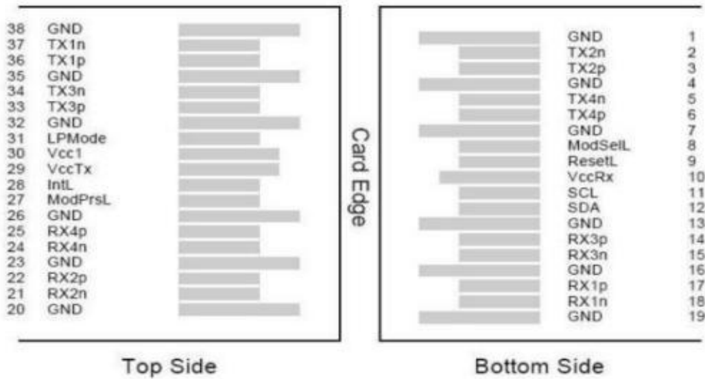
QSFP28 Transceiver Electrical Pad Pinout
