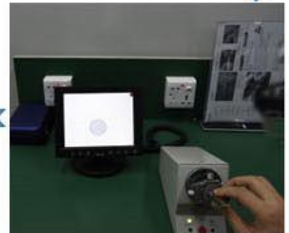
Cleaning end face
