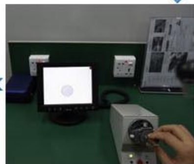
Cleaning end face
