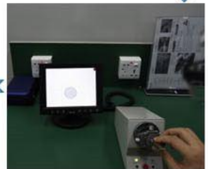
Cleaning end face
