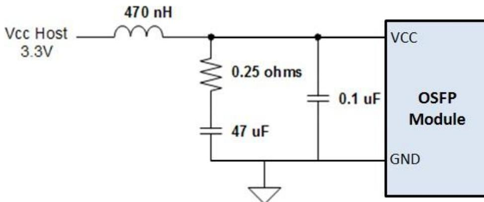
Figure 5. Recommended Power Supply Filter
